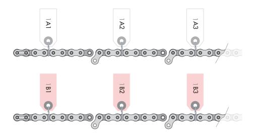
The tags fitted to the chains indicate in which position/order the chain should be installed:
