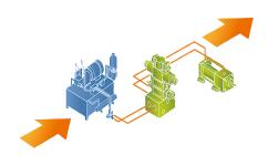
Goods transported by a conveyor can be sorted into multiple levels by high-speed lifting, realizing a reduction in vertical transport time.
