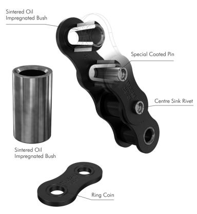
Fig. 10 Basic Construction
