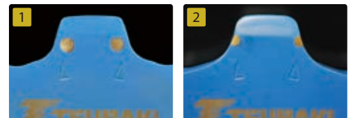
Comparison – New (1) vs. Worn Sprocket (2)
