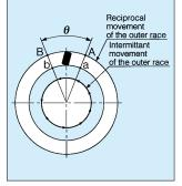
(of the driven side) does not rotate. By repeating this sequential movement, the inner race (of the driven side) rotates intermittently within the preset angle ( $\theta$ ).
