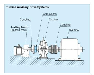
This example shows a Cam Clutch installed in the auxiliary drive system of a steam turbine. The auxiliary drive system powers the turbine at low speed through the engaged Cam Clutch, until steam pressure accelerates the turbine to the Cam Clutch release speed. Then the cam automatically disengages and runs as a high speed ball bearing, because there is no mechanical contact in the clutch.
