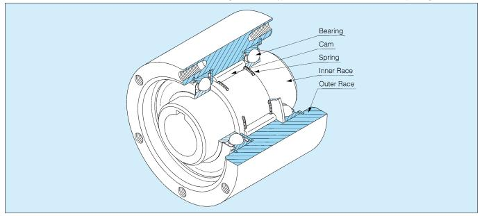
The figure shows a typical model from the MZ Series for explaining construction.
