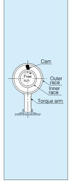
Prevention of reverse rotation of inclined and vertical conveyors is a typical example of how backstopping is used. The following A, B, and C types are available for different Cam Clutch mounting positions, and the series listed are designed to handle each specification.
